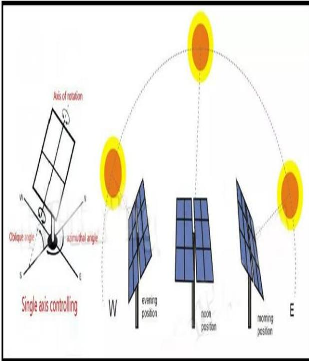
Figure 5: single-axis solar tracker
