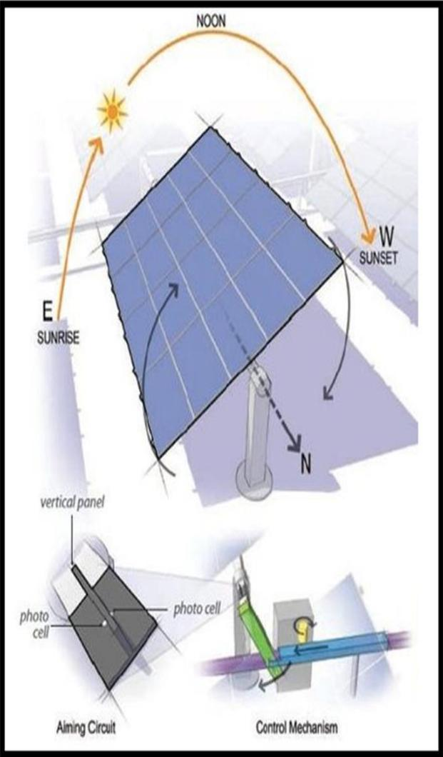
Figure 4: single-axis solar tracker
