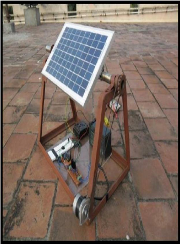
Figure 2: prototype of a single-axis solar tracking system
